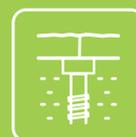
'Lost Head' hidden fixing using DuraFix stainless steel trimhead screws
