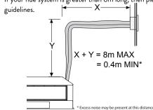
Horizontally Terminated: Utilises the Escea horizontal power flue enclosure kit
