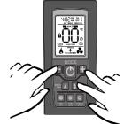
Now hold down the 'EDIT TIMER' and 'ACTIVATE TIMER' buttons simultaneously; the remote display will show the current configuration of either 'NG' for Natural Gas or 'LP' for ULPG/Propane. To change this configuration, hold down the 'EDIT TIMER' and 'ACTIVATE TIMER' buttons simultaneously for 5 seconds. This will now have toggled between gas types.
