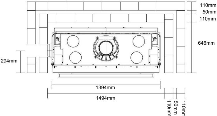
7.1 Side and Rear thermal insulation layers
