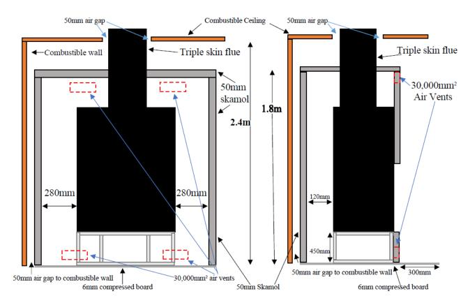
Minimum 7 sheets x 50mm Skamol board (2040 x 1220) for Chimney breast build out, extra required for extra caps reqruied on left and right for cabintry, and if taller cavity required or ceiling height is more the 2400mm.
