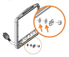
Close the door with the door handle to test for any improvement. If no improvement, remove second washer.
