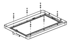
Gently lift the glass retainer up and out, taking careful note that the glass may still be held in the retainer and could fall out.
