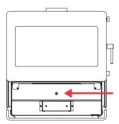
Slide the fan assembly outwards from the rear of the heater. When out, unplug the cable to disconnect the fan.
