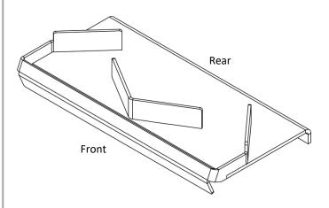
Installed the B800 baffle in the same method as described for the B500. Refer to image below for orientation of baffle plate within the firebox).
