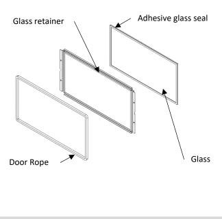
2.8. REPLACING THE DOOR SEAL
