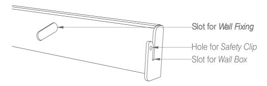
**NOTE:** After hooking the *Wall Box* onto the *Wall Hanger Bracket (Step 2)*, make sure that the *Safety Clips* (image below) supplied are fitted into the appropriate holes to prevent the Wall Box from accidentally becoming dislodged from the wall.
