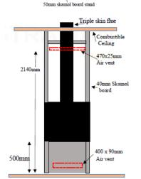
CLEARANCES BASED ON INSTALLATION HAWKWIND 200MM TRIPLE SKIN FLUE KIT. UNIT TO BE PLACED ON A BOX 1000MM[w] x 400MM[h] x 470MM[d] MADE FROM 50MM SKAMOL
