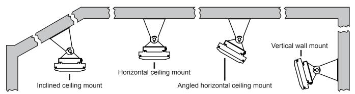
The ideal mounting position is directly above the area to be heated with a longitudinal orientation and facing vertically downwards. If this is not possible, the heater(s) can be mounted on a wall and angled downwards. For this application ensure the mounting height is within 2.1m to 2.7m.
