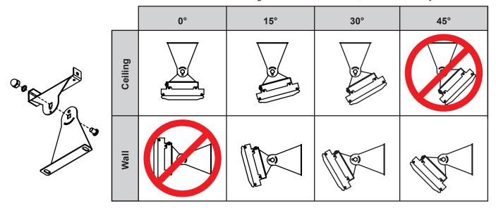
4. Mark the position of the two brackets, using the following minimum recommended bracket spacing below to determine the correct location.
