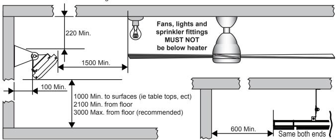
Minimum clearances when mounting the heater parallel with A CEILING.
