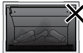
SOOT BUILD UP
