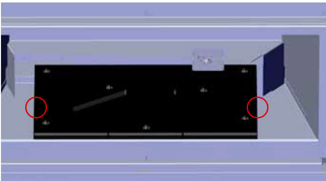
Diagram 2 - Burner Screw Locations
